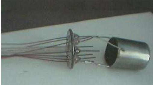
fig. 2. Factory glass wafer (8 pin for octal tubes)
