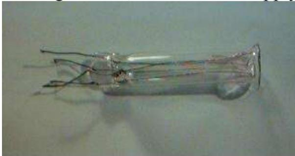
fig.4. glass-metal connector with for wires
