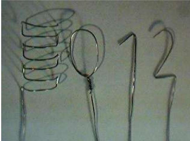
**fig.5. The electrodes**
