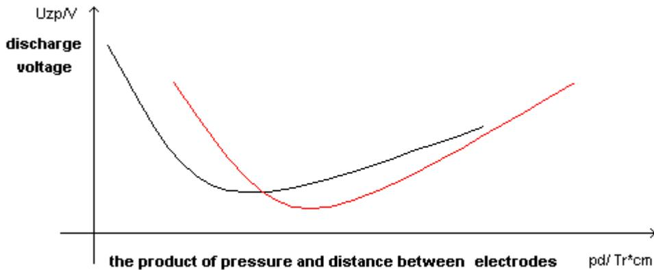
Fig.3. The Paschen's curves. Black curve for pure neon, red curve for 99% neon and 1 % argon
